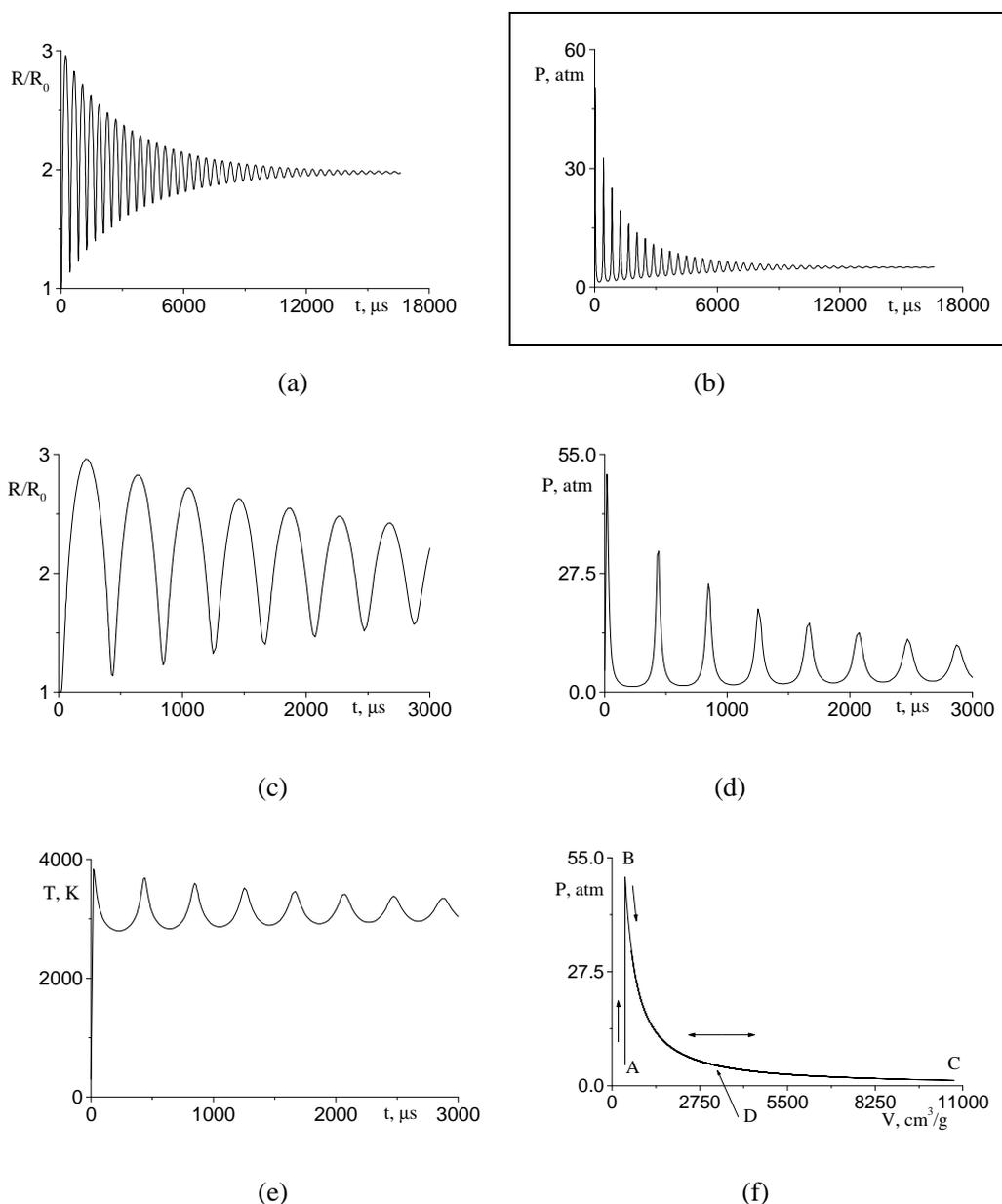
**Fig.4 Bubble dynamics and gas parameters after ignition**
