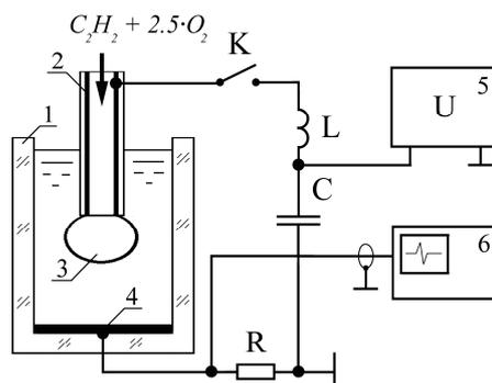
1–Plexiglas cavity; 2–tube-electrode; 3– bubble with the acetylene–oxygen mixture; 4–opposite electrode; 5– unit for charging the capacitor C; 6– digital oscillograph; electromagnetic switch is denoted as S, Parker’s shunt as R, and inductance as L.
