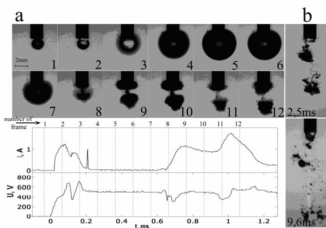
**Fig.2 (a) Frames of one cycle of burning of the acetylene–oxygen bubble in water correlated with the electrical parameters of current and voltage; (b) subsequent fragmentation of bubbles; frame rate 104 frames/sec**
