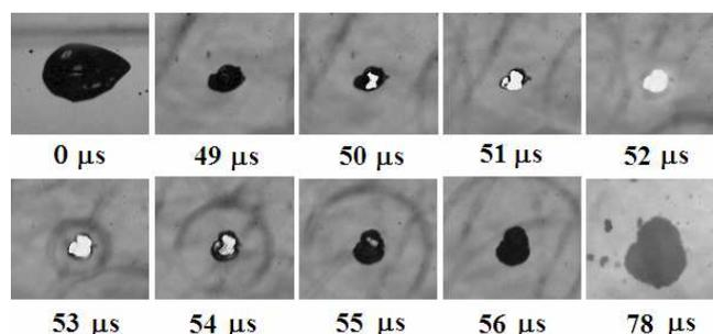
**Fig.3 Shock induced explosion of a single bubble and subsequent emission of acoustical waves. Oxygen bubble in cyclohexane. The incident shock wave exerts impact on the walls of the bubble at  $t = 0$  (experiment [5], see also [6, 7])**
