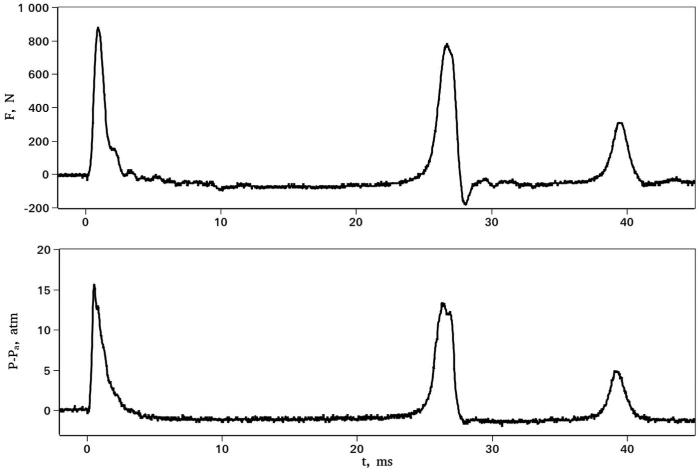
Fig. 2. Synchronously recorded oscillograms of force impulses  $F(t)$  and pressure pulses  $P(t)-P_a$ .
