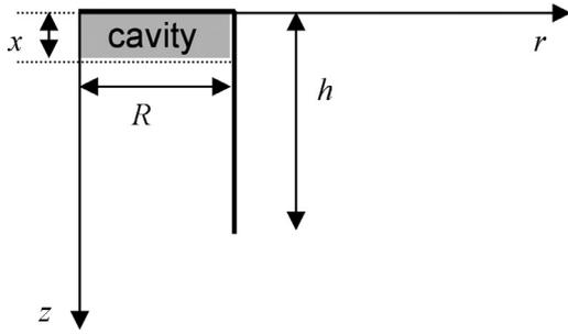
Fig. 4. Mathematical formulation of the problem of cavity pulsation in a cylindrical chamber.
