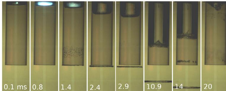
Fig. 3. Shadowgraph of the dynamics of the processes inside and outside the chamber for a gaseous charge with  $V_0=3$  ml,  $d=29$  mm, and  $h=83$  mm.
