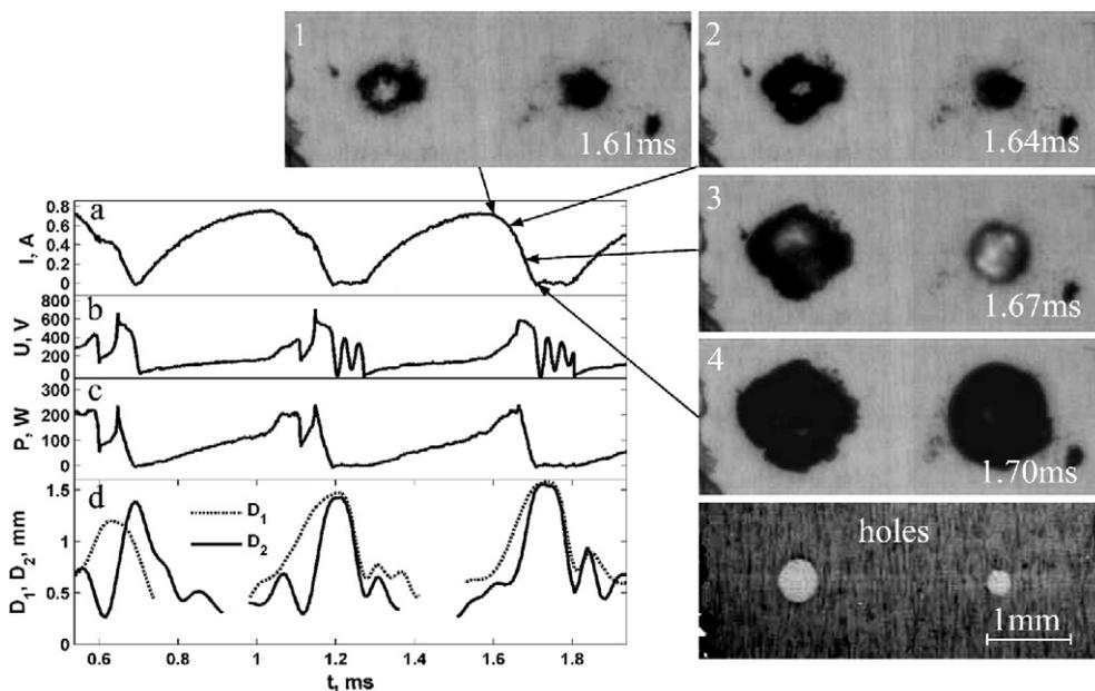
Fig. 3. Frames of high-speed recording and corresponding oscillograms of current (a), electrode voltage (b), released power (c), and plot of bubble edge motion (d) for self-oscillations on concentrators of setup 2 ( $d_1 = 0.45$  mm,  $d_2 = 0.25$  mm).  $L = 30$  mH,  $U_C = 200$  V.
