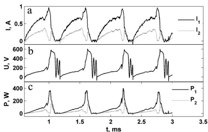
**Fig. 4.** Current oscillograms on concentrators (a), electrode voltage  $U$  (b), and released power (c) for the experiment of setup 3 ( $d_1 = 0.45$  mm,  $d_2 = 0.25$  mm).  $L = 30$  mH,  $U_C = 200$  V.
