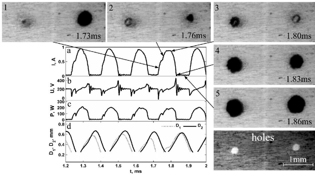
Fig. 2. Frames of high-speed recording and corresponding oscillograms of current (a), electrode voltage (b), released power (c), and plot of bubble edge motion (d) for self-oscillations on concentrators of setup 1 ( $d_1 = 0.25$  mm,  $d_2 = 0.26$  mm).  $L = 2.3$  mH,  $U_C = 200$  V.
