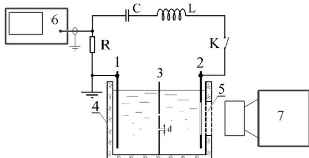
Fig. 1. Principal scheme of the experimental setup for the study of self-oscillations on two current concentrators in the form of holes in a dielectric film.
