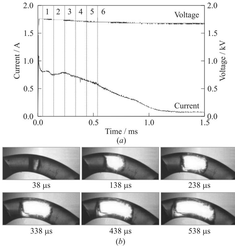
**Figure 3** Current and voltage oscillograms (a), and the frames that illustrate the dynamics of hydrodynamic processes during initiation of combustion of a propane–oxygen bubble (b)
