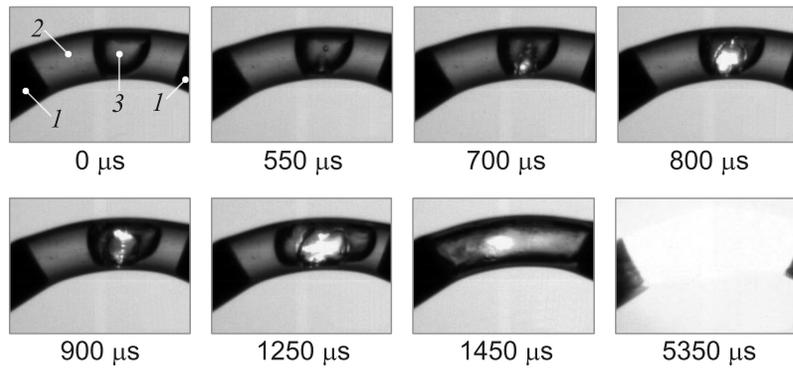
**Figure 2** Dynamics of the electric explosion of a thin electrolyte layer on the boundary with an air bubble ( $U = 1200$  V): 1 — tubular electrodes  $d = 2.5$  mm (the positive and negative electrodes are located on the left and on the right, respectively); 2 — electrolyte, 1% NaCl solution in water; and 3 — air bubble
