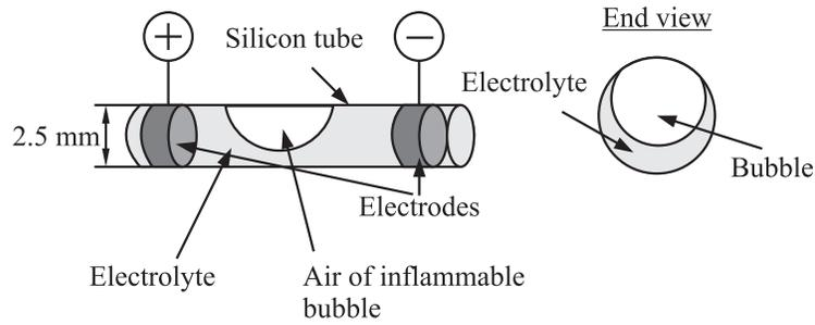
**Figure 1** The arrangement of the experiments
