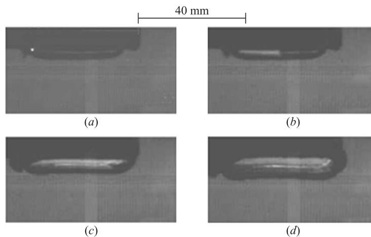
**Figure 2** Speed-recording frames of the process of combustion and beginning of quasi-cylindrical bubble expansion: (a)  $98 \mu\text{s}$ ; (b)  $456 \mu\text{s}$ ; (c)  $965 \mu\text{s}$ ; and (d)  $1298 \mu\text{s}$
