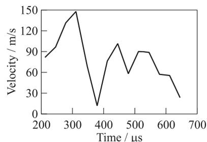
**Figure 3** Diagram of combustion front velocity for mixture  $C_3H_8 + 5O_2$  in a quasi-cylindrical bubble
