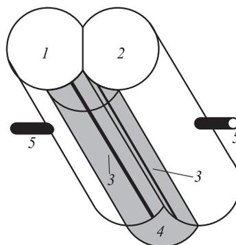
**Figure 1** The scheme of linear-slot injector for gas combustion in water in separate supply of gases into water: 1 and 2 — copper cylinders; 3 — slots; 4 — quasi-cylindrical bubble with combustible mixture (shown in grey color); and 5 — tubes for separate gas supply
