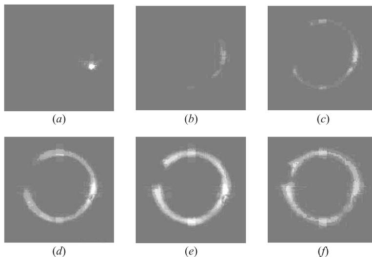
**Figure 4** Speed-recording frames of the process of combustion of propane–oxygen mixture in a circular bubble with ring 4 cm in axis diameter and gas volume is  $3\text{ cm}^3$ : (a)  $0\ \mu\text{s}$ ; (b)  $300$ ; (c)  $400$ ; (d)  $500$ ; (e)  $600$ ; and (f)  $700\ \mu\text{s}$ . (Refer color plate, p. XXX.)
